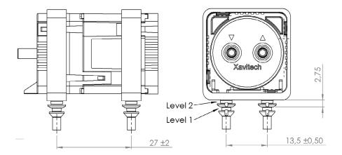
Drill hole 4 x Ø3 mm for level 1 mounting
