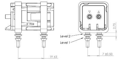
Drill hole 4 x Ø3 mm for level 2 mounting Drill hole 4 x Ø2mm for level 1 mounting
