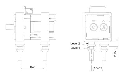
Drill hole, level 2: 3.5 mm Drill hole, level 1: 3.0 mm
